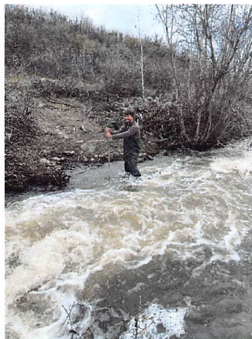
Figure 3: Measuring streamflow on Cache Creek – 2023
