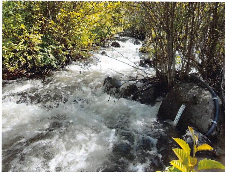
Figure 2: Staff gage and Pressure Transducer Housing.
